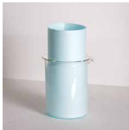
Fig. 20 Immersion of a shaped paper in a test liquid
