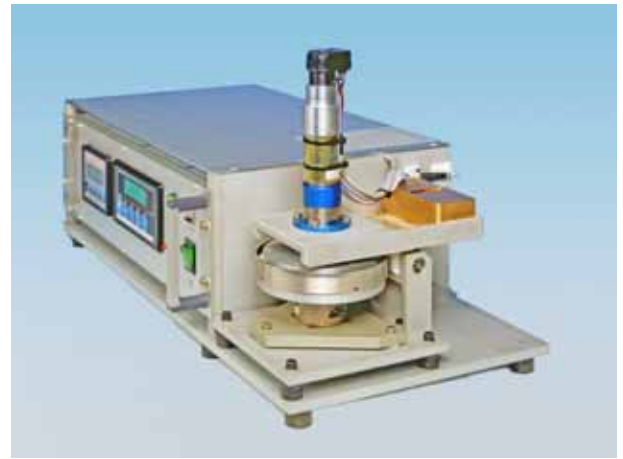
Fig. 08 ... and once again the Rotation Wiping Simulator in use
