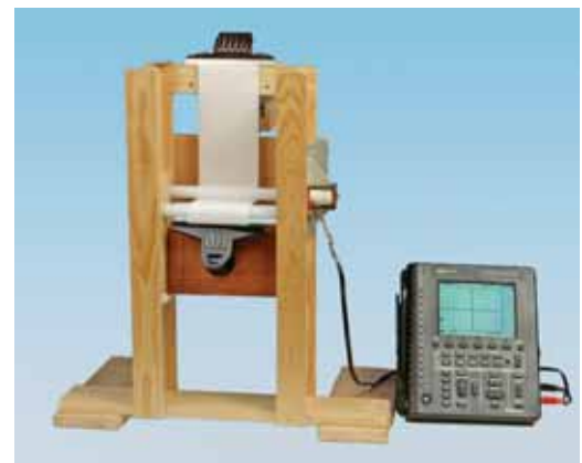
Fig. 27 Triboelectricity drop sledge after Ehrler and oscilloscope
