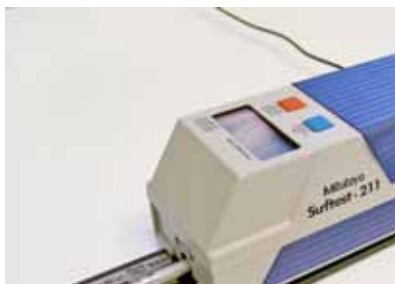
Fig. 04, 05 Surftrons measuring device for surface roughness, left with calibration standard,
