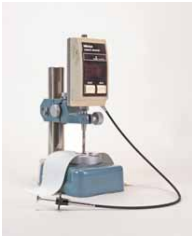
Fig. 01 Electric thickness gauge. For fabrics and paper, Mitutoyo
