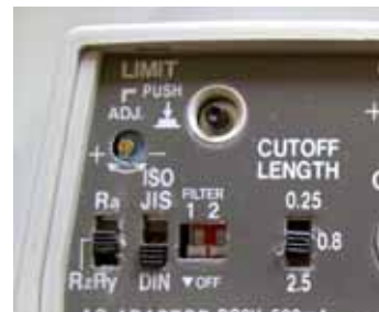
Fig. 04, 05 Surftrons measuring device for surface roughness, left with calibration standard,
