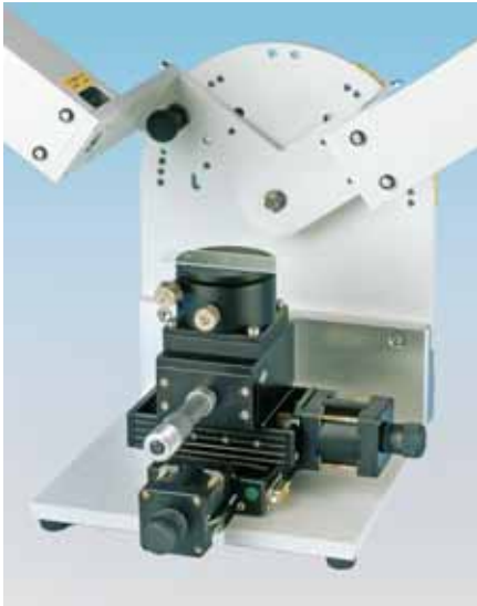
Fig. 34 Riss-Ellipsometer to measure the thickness of extremely thin, transparent contaminant layers in the nm range (examples Fig. 35, 36)
