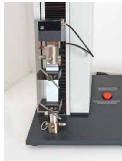
Fig. 03 Maximum tensile strength / expansion gauge, Adamel
