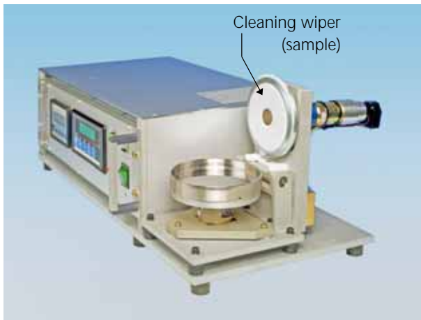
Fig. 07 Labuda Rotation Wiping Simulator Mark II for testing particle attrition (in opened state)
