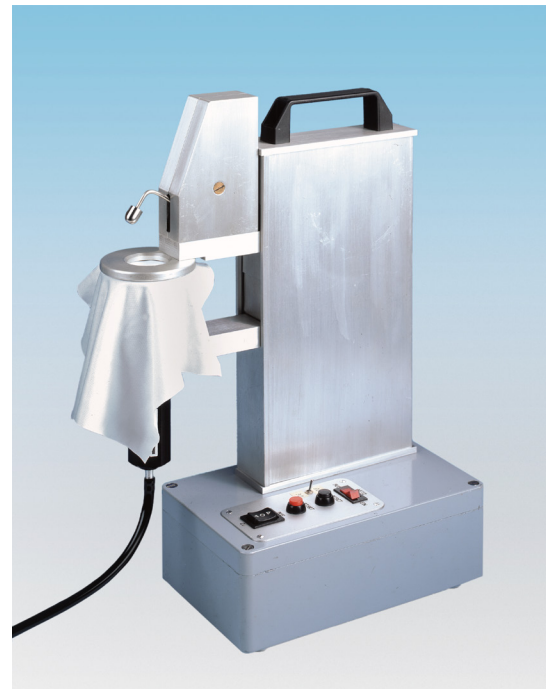
Fig. 14 Ball-Hammer Testing Device after Labuda
