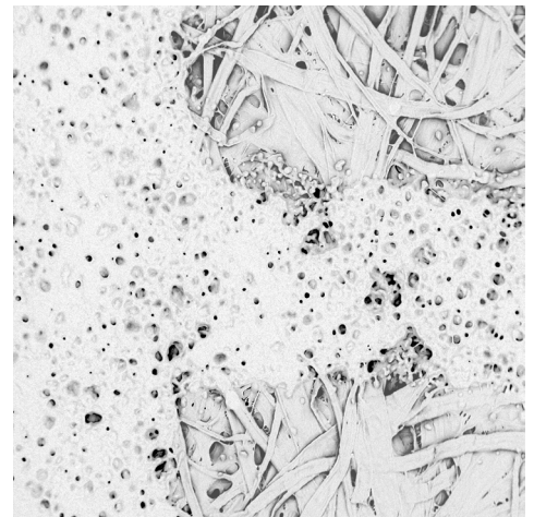
Fig. 21 Toner printing, laser: letter E on pure paper Galaxy®
