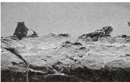
Fig. 19 the edge of paper 4 is quite even and therefore on a higher quality than the specimen formerly tested.
