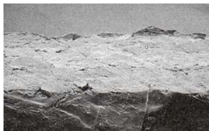
Fig. 20 paper 5 shows a clean cut, without any loose fibres or particles
