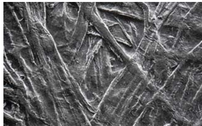
Fig. 8 Paper 5 - homogenous distribution of the fibers. Here the Latex-finish is evenly applied.
