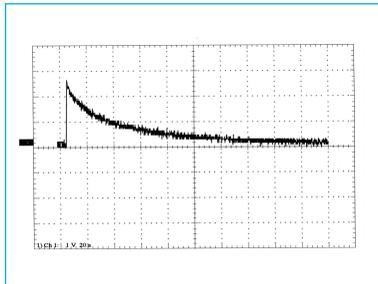
**Fig. 13** Standard charge diagram. PES knit, washed (+ 8638 V: 195 s)
