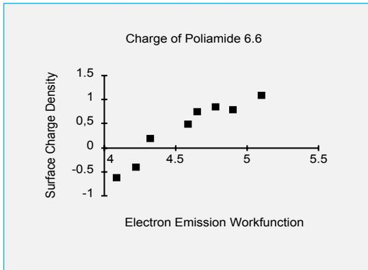
**Fig. 2** R.G. Arridge drew this well-known diagram about surface charge density in elementary charges per surface unit relative to the electron workfunction of various metals WM. We can assume from it that e.g. the electron workfunction for poliamide 6.6 is about 4.4 eV.
