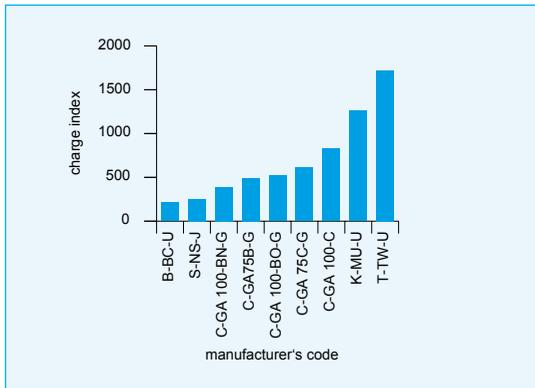
Fig. 30 Charge index for various cleanroom *papers*
