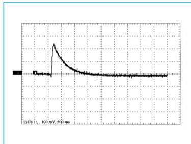
**Fig. 17** Charge diagram, standard cleanroom paper with polymer coating (+796 V: 1,43 s)
