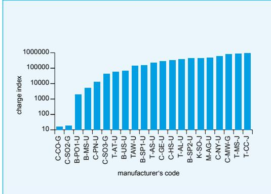
Fig. 29 Charge index for various cleanroom *knit wipers*
