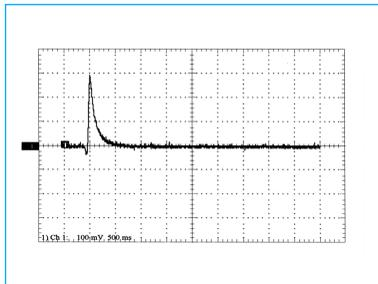
**Fig. 16** Charge diagram, the same material as in Fig. 15, but half of the sample wet (+938 V: 750 ms) (enlarged to a scale of 1:5)
