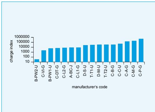
Fig. 31 Charge index for various cleanroom *nonwoven wipers*
