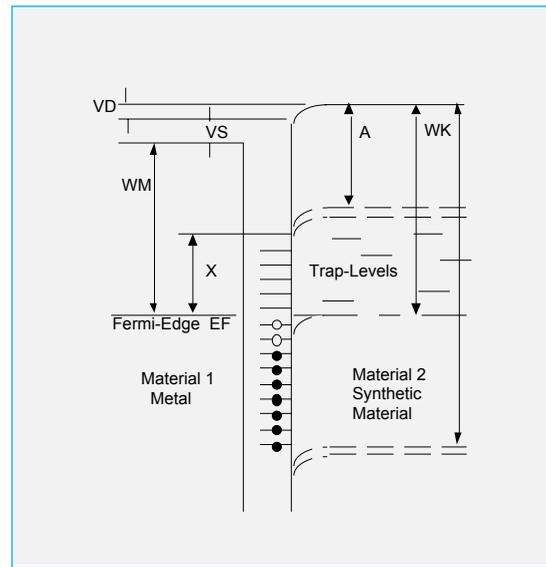
**Fig. 1** Energy diagram of the charge-transfer after Bauser. Meaning of the indices:  $W_1$ ,  $W_2$  - workfunction of the two materials 1 and 2;  $I$  - ionization energy;  $A$  - electron affinity of material 2;  $EF$  - Fermi level
