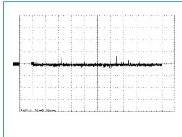
**Fig. 14** Comparison to Fig. 13: Charge diagram, PES-knit, moistened with deionized water (no charge, 0 V: 0 s)
