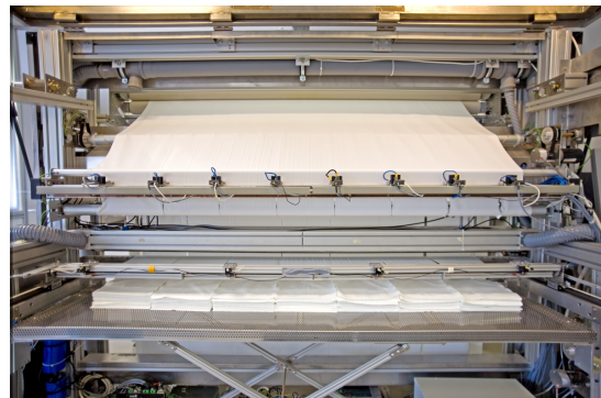
Fig. 14 Formatting and stacking station with automated wiper stacking and laser formatting
