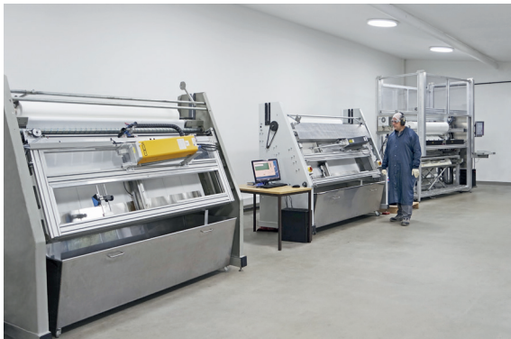
our laser formatting for knit wipers
